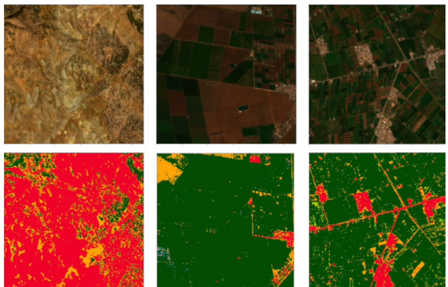
Illustration of pixel classification with 3 visible classes of pixels (Copernicus Sentinel data 2019)
